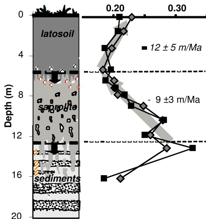
**Figure 1** Propagation rate of a weathering front determined by  $^{238}\text{U}$ - $^{234}\text{U}$ - $^{230}\text{Th}$  disequilibrium method in a lateritic profile developed on sediments (Manaus, Brazil) (in. Pelt, PhD Thesis, 2007). Black squares: ( $^{230}\text{Th}/^{232}\text{Th}$ ) activity ratios; grey diamonds: ( $^{238}\text{U}/^{232}\text{Th}$ ) activity ratios.
