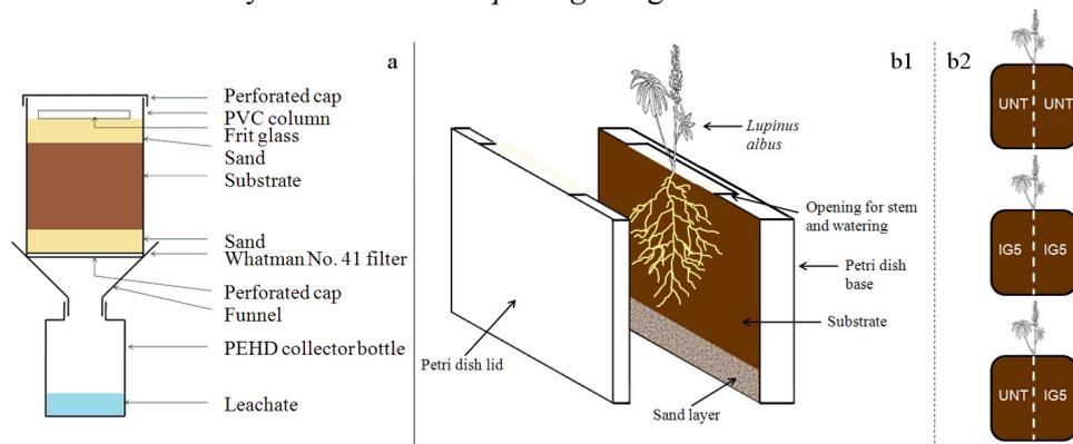
**Figure 1. Design of the leaching column (a) and rhizobox (b1) and experimental designs (b2).**
