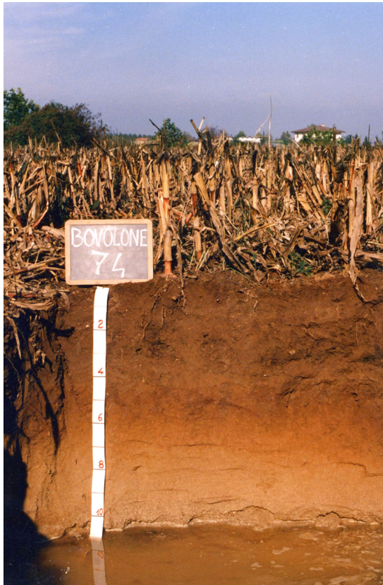
Figure 3. Soil profile exhibiting distinct vertical spatial patterns. Below the O horizon where the plant debris accumulates (few centimeters thick), there is the plough layer, rich in humus (Ap horizon, up to about 30 cm), followed by the well-structured cambic B horizon (25 cm thick) and the reddish BC horizon, until 70 cm. The parent material is made of light brown fluvial sands. The groundwater fluctuates at about 110 cm depth. Every horizon offers different spatial and temporal boundary conditions to soil biodiversity and its functionality.
