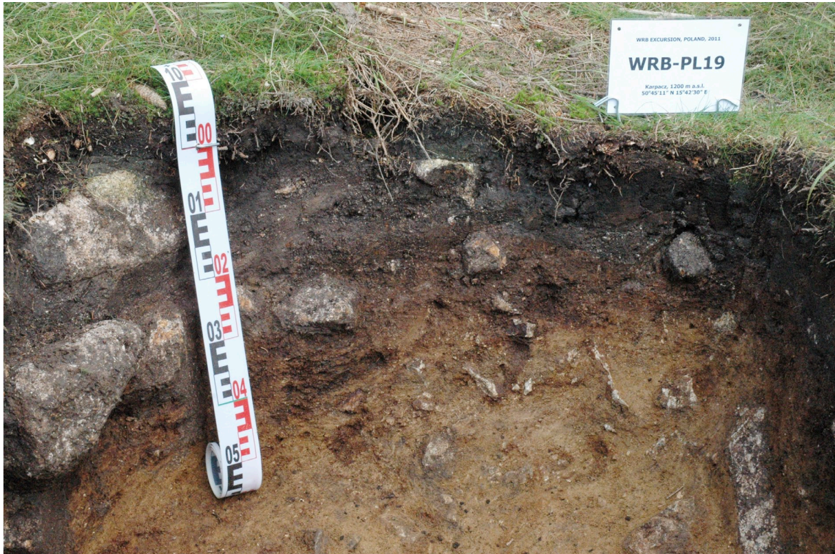
Figure 1: WRB Classification according to the Guidelines 2010: Eutric Cambisol (Colluvic, Silty) over Haplic Luvisol (Cutanic, Hypereutric, Lamellic, Silty) .
