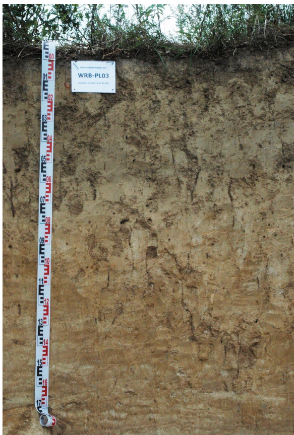
Figure 2: WRB Classification according to the Guidelines 2010: Folic Albic Podzol (Oxyaquic, Ruptic, Skeletic) .
